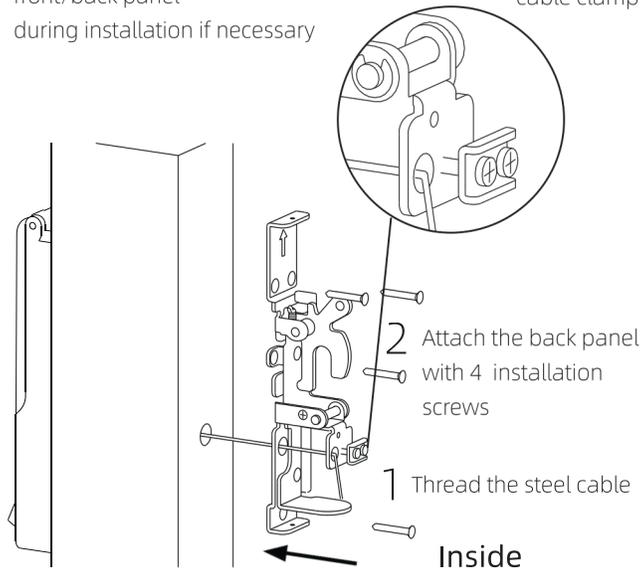
Step 4: Fix the steel cable
