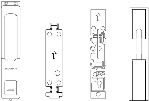
1. Front panel    2. Front panel mounting plate    3. Back panel    4. Back cover mounting plate
